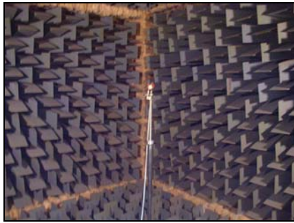
Fig. 5 The anechoic test chamber is triangular. No two surfaces are parallel, thus ensuring a reduction in standing waves. A Brüel & Kjær 1/2" Microphone Type 4191 is used for measurement
