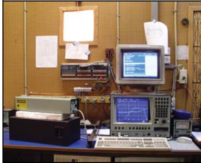
Fig. 4 Peerless' lab uses Brüel & Kjær Audio Analyzer Type 2012. The unit on the right is Laser Velocity Transducer Type 8323, used to measure the velocity of a loudspeaker's diaphragm
